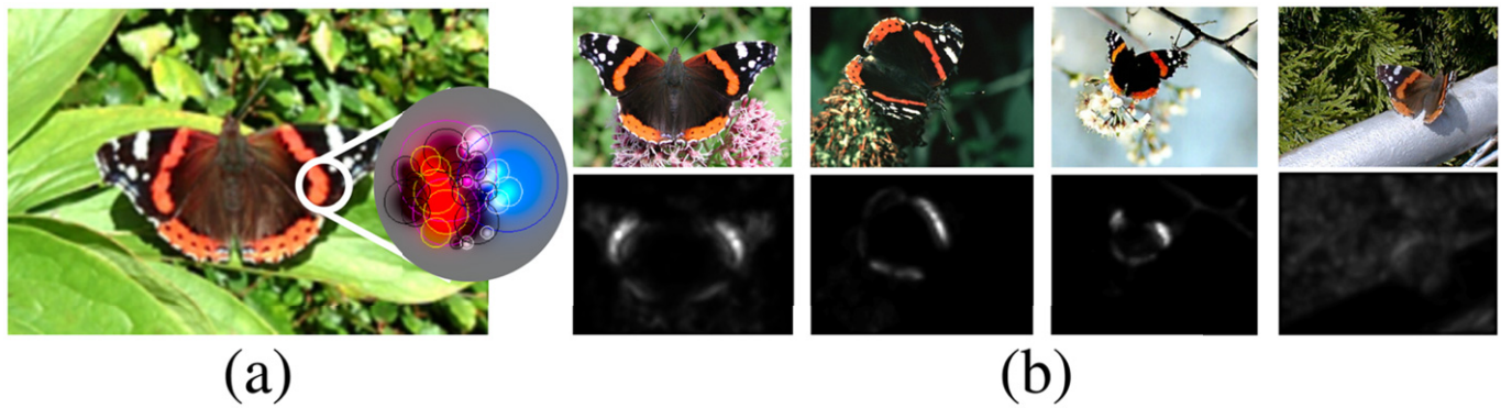
Fig. 8. (a) Configuration of a part-selective COSFIRE filter with the encircled pattern from a training butterfly image. The inset shows the structure of the resulting filter. (b) Butterfly test images (top) and the corresponding response maps (bottom) achieved by the configured filter with rotation and scale tolerance.
